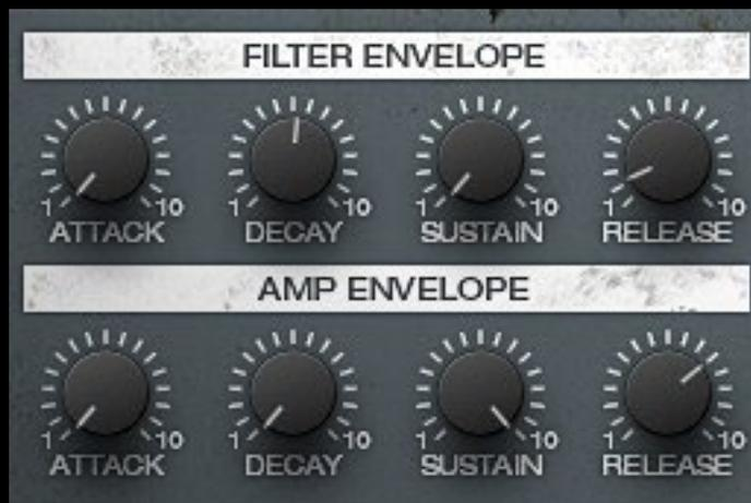
Both envelopes have separated functions, the filter envelope can modify, as the name already suggest, the lowpass filter - controlled by the „Env Mod“ inside the filter section.
