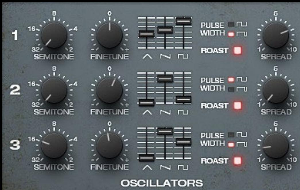
The oscillator section contains 3 oscillators, each of them generates 3 waveforms at once: triangle, sawtooth, pulse (with 50% or 90% pulsewidth).
