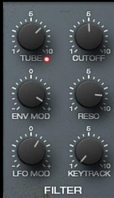
The filter section gives you access to the great sounding 4-pole ladder lowpass filter unit. Main controls for the filter are: Cutoff, Resonance and Keytrack.
