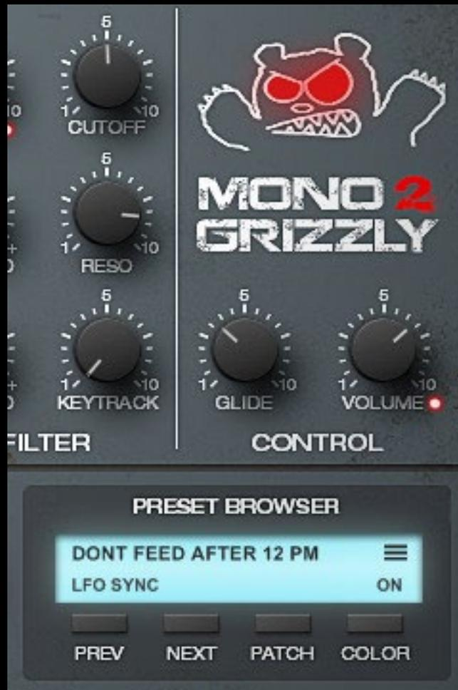
On the right side of the MonoGrizzly you have access to the preset browser. Here you can step through the presets by using „Prev“ & „Next“. By clicking on the 4-line symbol the preset list will show up. You can also rename presets with right-mouse-click on the preset name. The button „Patch“ opens the menu for loading and saving single presets and preset-bank.
